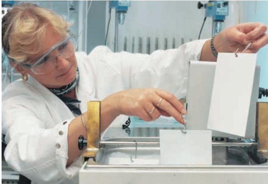
*Performance of a caustic soda detergent test at BASF Coatings AG.*
