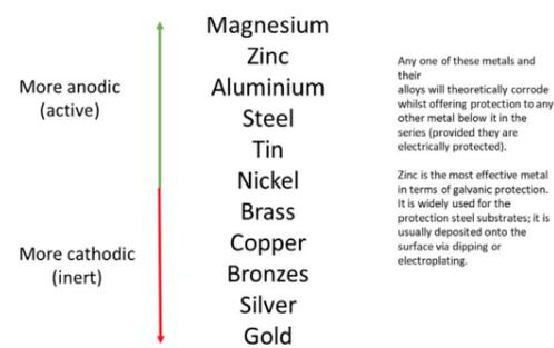
Any one of these metals and their alloys will theoretically corrode whilst offering protection to any other metal below it in the series (provided they are electrically protected).
