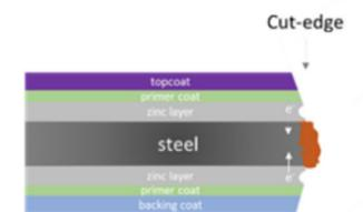
Zinc (more anodic than the steel) sacrificially corrodes to protect the steel substrate. Electrons ( $e^-$ ) flow from the zinc to the steel. Once the zinc in the vicinity of the cut-edge is depleted, the steel starts to corrode and produces red rust.
