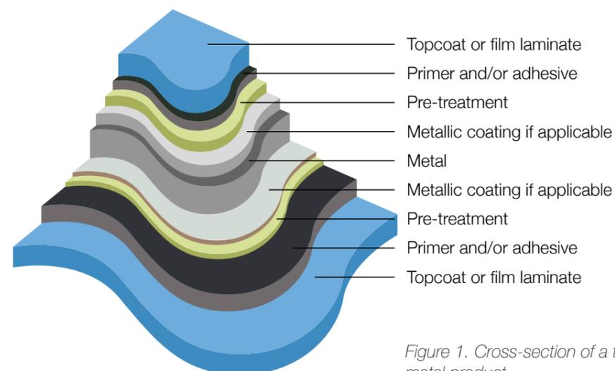
Figure 1. Cross-section of a typical prepainted metal product
